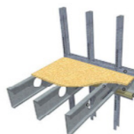
SF 140 or 190 Joist to LGSF Wall C
