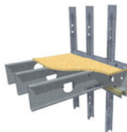
SF 240 or 290 Joist to LGSF Wall B
