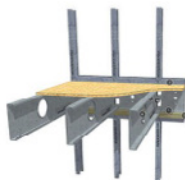
SF 140 or 190 Joist to LGSF Wall D
