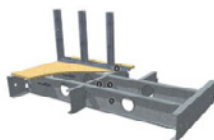
SF Joist Blocking Standard Detail
