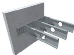
SF Joist to Concrete Wall
