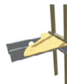
Speedfloor Steel Joist Ext Wall Bracket Detail
