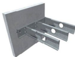
SF Joist to Concrete Wall
