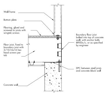
Joist to concrete or block walls
